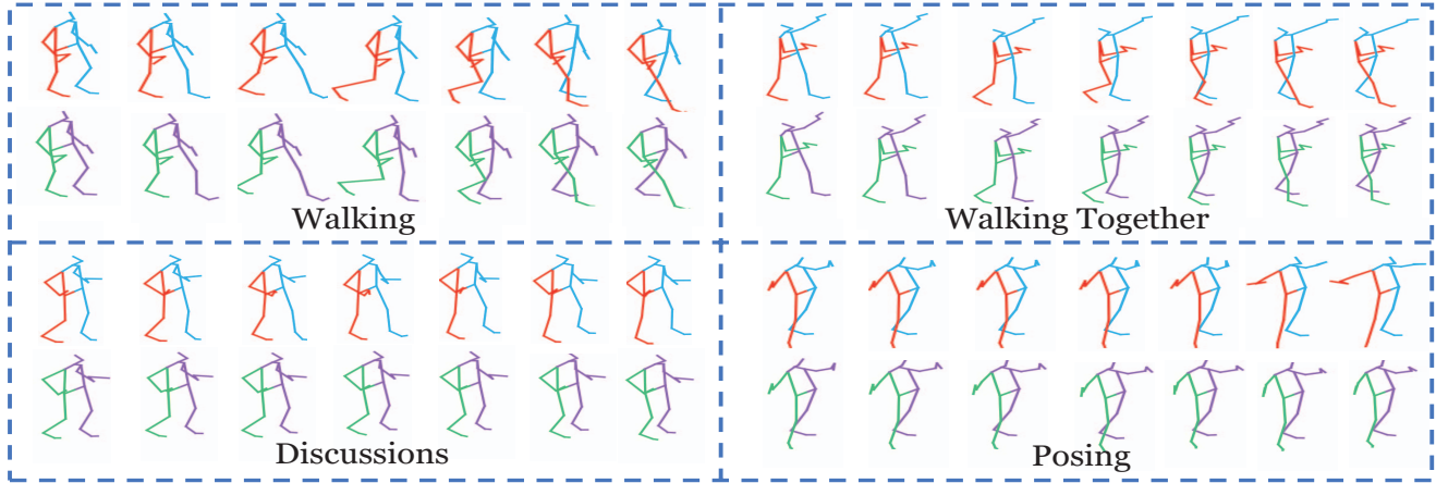
Figure 3. Visualization of predicted sequences against Ground Truth sequences for 80, 160, 320, 560, 720, 880, 1000ms. We demonstrate the prediction of "Walking", "Walking Together", "Discussions", and "Posing", where the green and purple lines indicate prediction and the red and blue lines indicate the corresponding Ground Truth.
