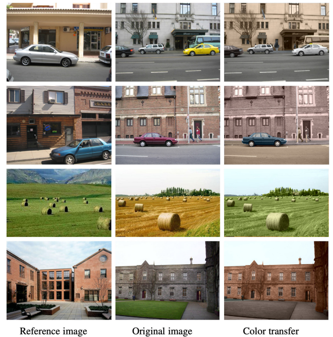
Fig. 15. Application of region correspondences. Changing the colors of the objects in the original image using the colors of the reference image.
